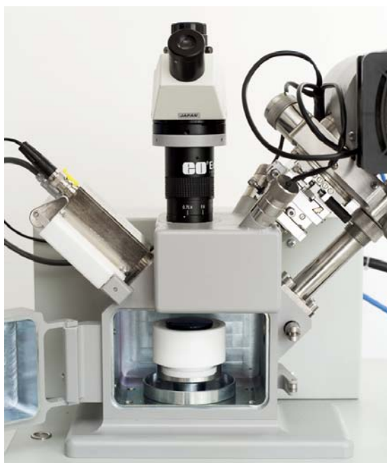
Fig 1. Optical lay out of Unisantis XMF–104 Micro Analyser
